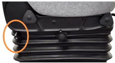
National HP & Bostrom Wide Ride II suspension style belt bar. Does NOT require use of lock nut (item 14).
