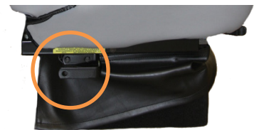
Bostrom T Series style belt ICP bracket. DOES require use of lock nut (item 14).
