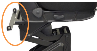
National 95 suspension style belt bar. Does NOT require use of lock nut (item 14).
