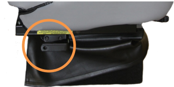
Bostrom T Series style belt ICP bracket. DOES require use of lock nut (item 14).
